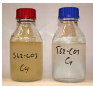
Figure 1: Example of water quality improvement between conventional valve (left) and Typhoon Valve System (right)
