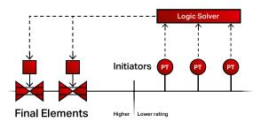
Mokveld is your single point of contact for the supply of an integrated HIPPS. Supplying only the certified valve / actuator combination (the final element) is also an option, for integration into the SIS by yourself or by others.
