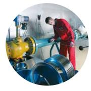
High-pressure flow facilities Unique R&D high-pressure flow facilities are available for noise testing of innovative valve solutions
