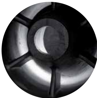
View through un-machined body casting showing ribs and inner-body
